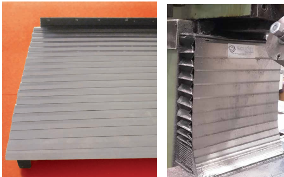
Example of bellow with stainless steel strips recommended for areas with hot shavings
